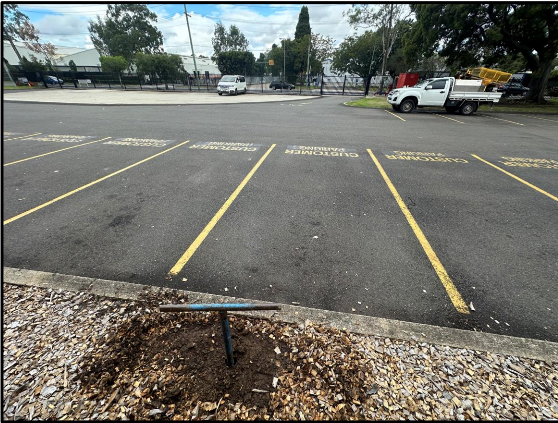
Figure 14. Sampling of BH10 using hand auger(6/5/2024).
